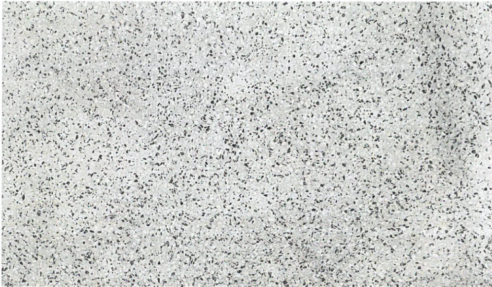
Fig. 1: VZ030230009 – Blasted terrazzo tiles
