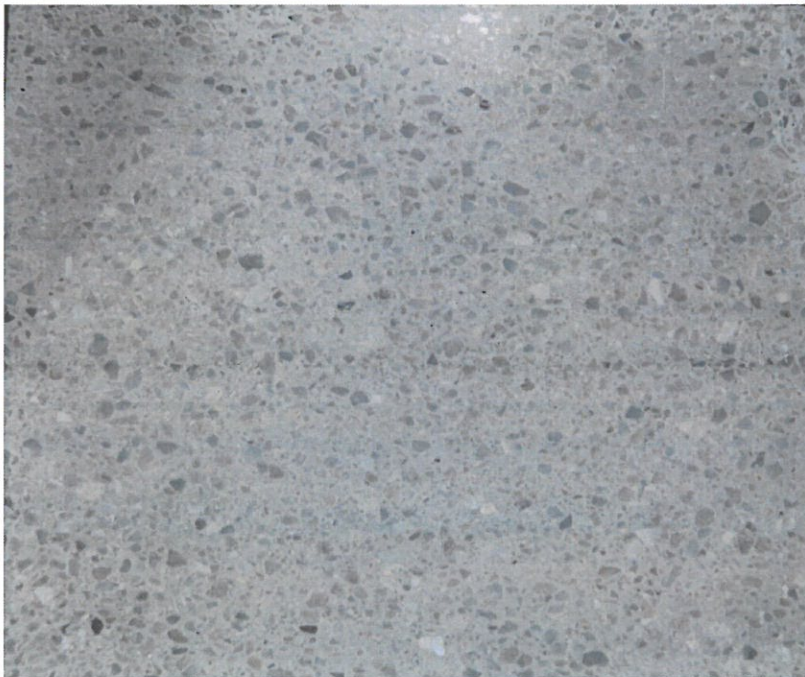
Fig. 1: VZ030210013 - Concrete elements with terrazzo surface
